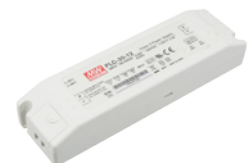
LED-DR30-12 12V DC Class 2 hardwire power supply 100-240V AC input, 1-30W 6-1/4"L x 1-1/4" H x 1-3/4"W c/UR/us Recognized for dry locations Can be used with AL-PWM-6A dimmer which consumes 3 watts
